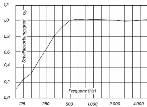
Schallabsorptionsgrad - Oktav-Mittenfrequenz
