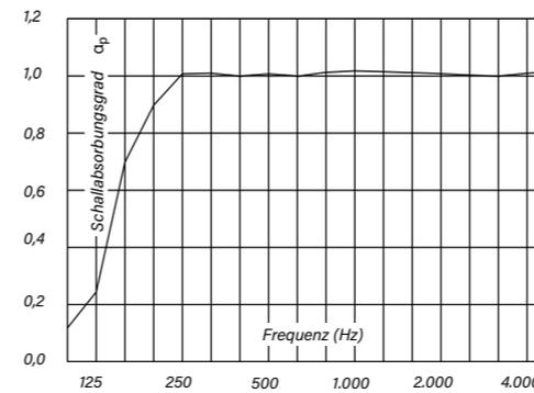
Schallabsorptionsgrad - Oktav-Mittenfrequenz
